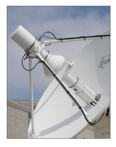
For program tracking only, TCS offers feeds in many frequency ranges from UHF & VHF through the Ku Bands. We have one design that operates in L-, S-, and X-Band as a single unit. This feed makes our Model 2400M Systems easier to deploy and maintain.
